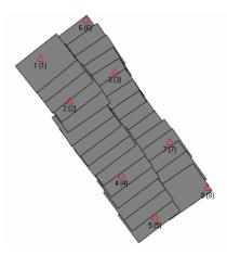
Figure 7. Block of 30 images taken at 760m flying height showing the distribution of ground control
