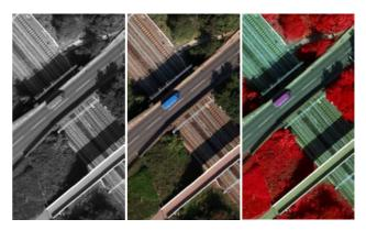
Figure 3. Panchromatic, colour and colour infrared images (Copyright Simmons Aerofilms Ltd)
