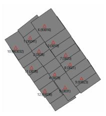
Figure 8. Block of 24 frame camera photographs taken at 880m flying height showing the distribution of ground control
