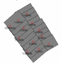
Figure 6. Block of 18 images taken at 1500m flying height showing the distribution of ground control
