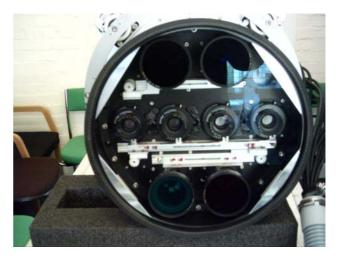
Figure 2. Multiple lens cones; 4 panchromatic across the centre and 4 larger colour cones (Copyright Simmons Aerofilms Ltd)
