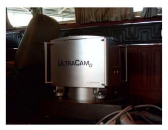
Figure 1. The Simmons Vexcel UltraCam D digital camera (Copyright Simmons Aerofilms Ltd)
